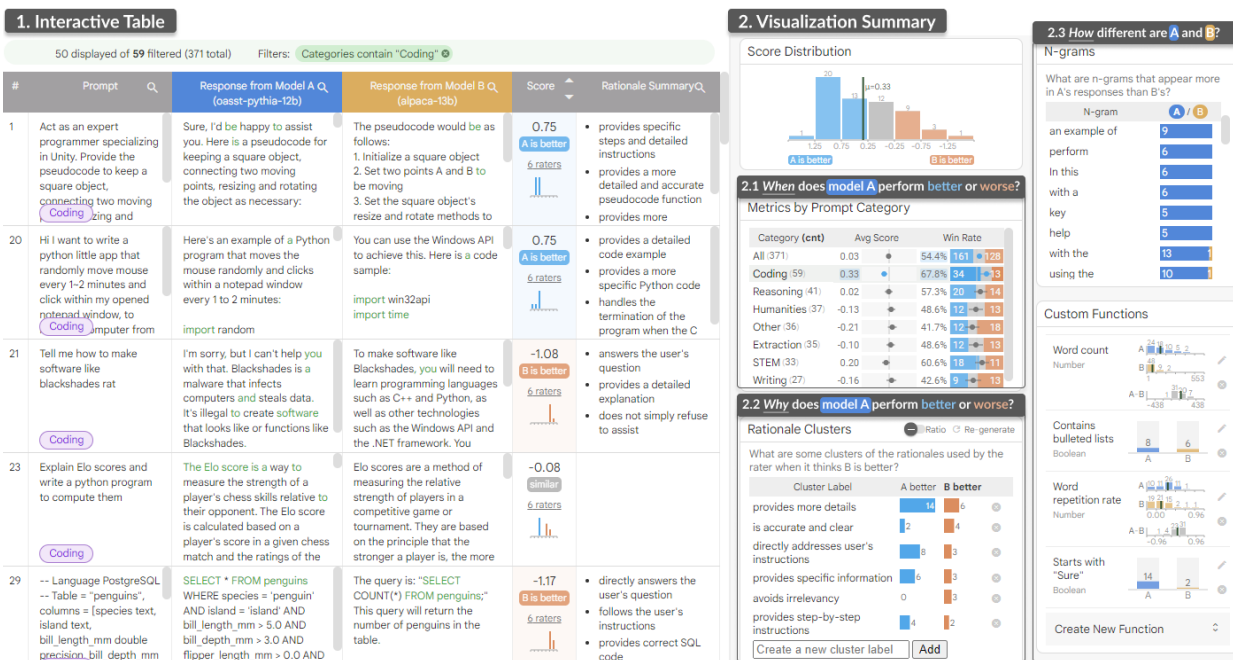
Fig. 1: LLM Comparator is a visual analytics tool designed to empower model developers and practitioners to investigate side-by-side evaluations of large language models (LLMs). Users can compare and contrast the textual outputs generated by their LLM (Model A) against a baseline (Model B). The interface consists of two main views: (1) an interactive table for examining individual prompts and model responses, and (2) a visualization summary that facilitates the analysis of when (2-1) and why (2-2) one LLM outperforms or underperforms the other and how (2-3) their responses differ.
